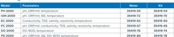
Meter comes with integrated electrode holder and universal power adapter (with six plugs). Kit option adds on electrode(s) or probe(s), BOD stirrer (for DO and PD only), and calibration solutions.
